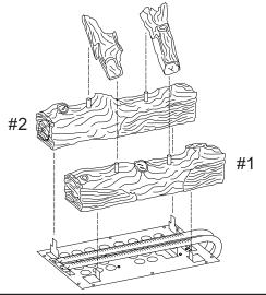
WARNING: Failure to position the parts in accordance with these diagrams or failure to use only parts specifically approved with this heater may result in property damage or personal injury.
